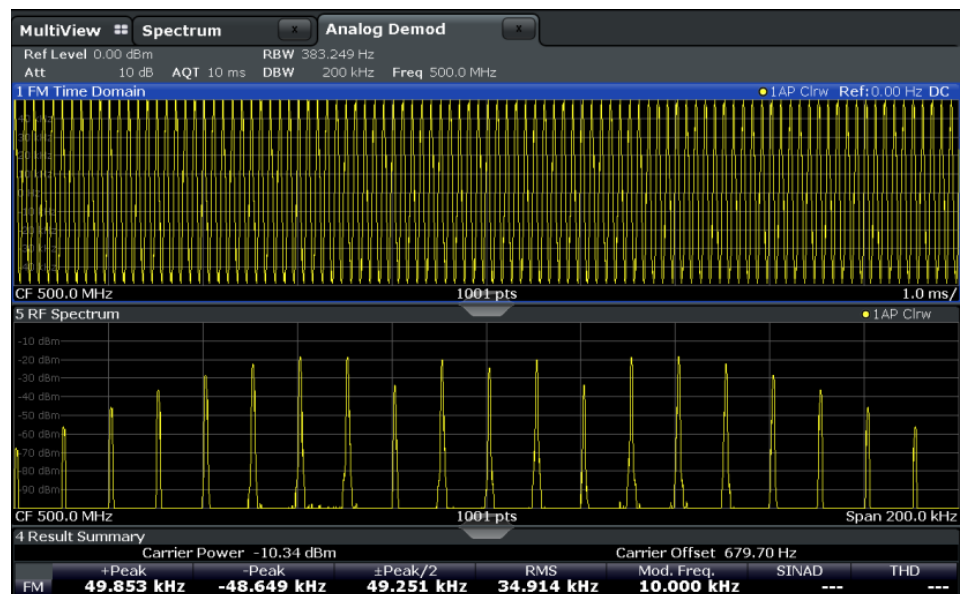
Fig. 8-4: RF spectrum with demodulation bandwidth = 200 kHz
